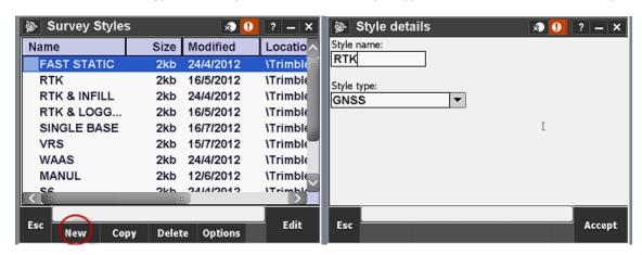
3. Now we need to setup the Survey styles to match the receivers and radio you're using. Options first.
